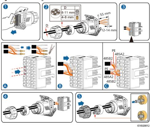
Figure 5-28 Installing the cable
