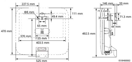
Figure 4-6 Mounting bracket dimensions
