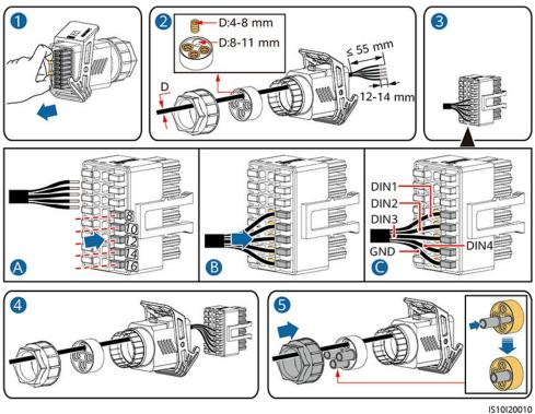
Figure 5-31 Installing the cable
