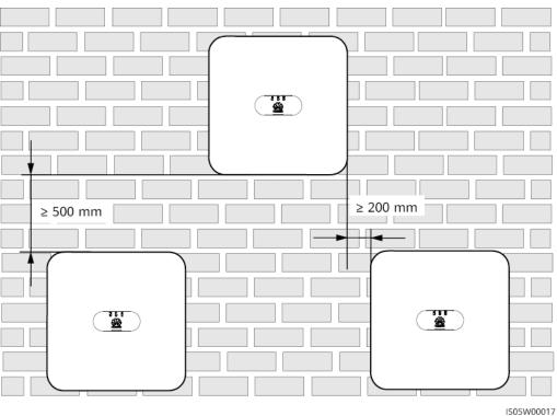
Figure 4-4 Staggered installation (recommended)
