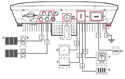
Figure 5-1 SUN2000 cable connections (optional in dashed boxes)
