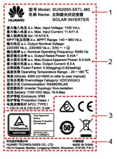
Figure 2-6 Nameplate (SUN2000-5KTL-M0 as an example)
