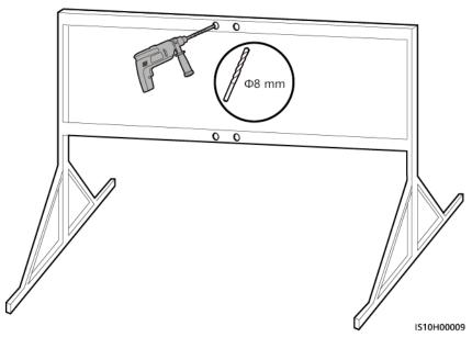
Figure 4-12 Drilling holes
