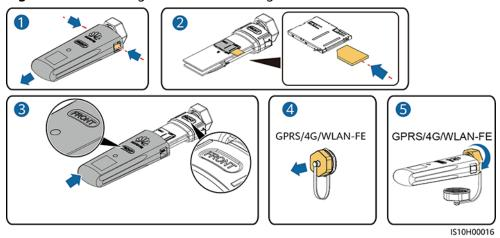
Figure 5-16 Installing the 4G Smart Dongle
