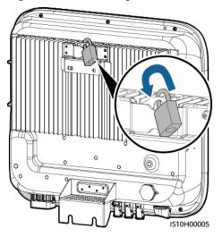
Figure 4-10 Installing the anti-theft lock
