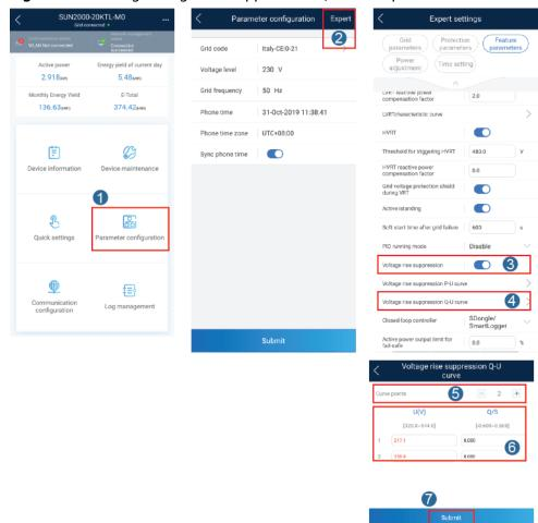
Figure D-1 Setting voltage rise suppression Q-U curve parameters
