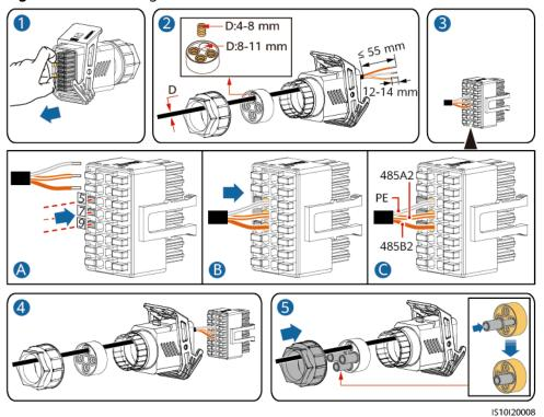
Figure 5-26 Installing the cable
